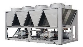
The Cooling efficiency of a chiller is expressed as its coefficient of performance COP or energy efficiency ratio EER which is the refrigeration capacity at full load (in Watts/ electrical input power (in Watts). Typically air-cooled chillers offer COP's in the range of 2.6 to 2.9
