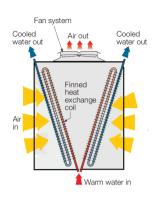
which for typical UK summer design conditions means that minimum cold water temperatures of between 35 °C to 38°C are possible.
