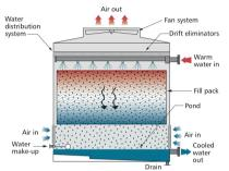
Water is cooled by evaporating a small proportion of the circulating water which causes the remaining water to be cooled. The evaporative process is highly efficient. Evaporative cooling towers are capable of cooling water to within 3 °C of the prevailing wet bulb temperature giving typical minimum cold water temperatures for the UK of 23 °C.
