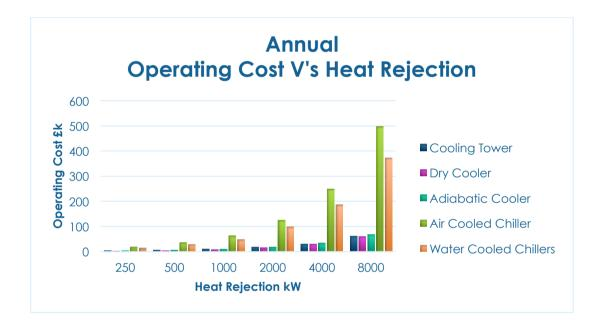
Comparing the operating costs for the air cooled chiller with the water cooled chiller the typical payback period in typically under two years.
