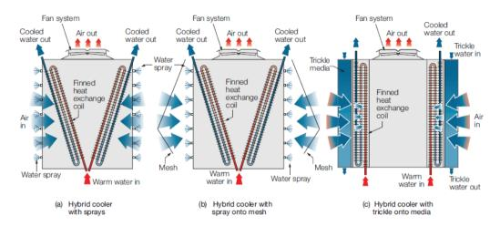
There are various designs of Adiabatic or hybrid cooler, which are basically dry coolers that have a spray or water trickle system to precool the air prior to it reaching the coil through which the cooling water flows. Precooling of the air is only required at higher ambient temperatures so for much of the time the unit operates as a standard dry cooler.
